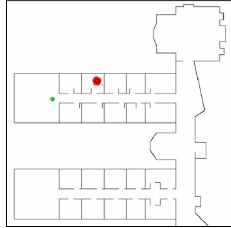
Fig. 26. Initial gaussian belief for robot 2 ( \sigma = 0.2 ).
