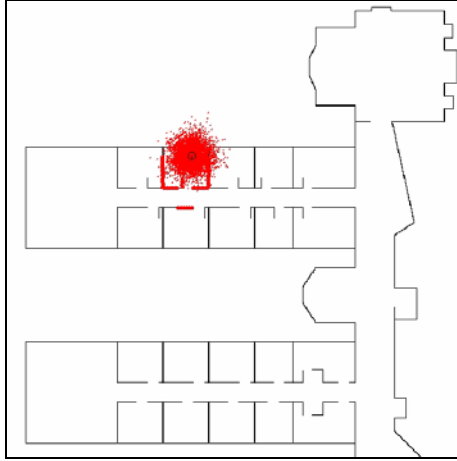
Fig. 24. Initial gaussian belief for robot 2 ( \sigma = 0.8 ).
