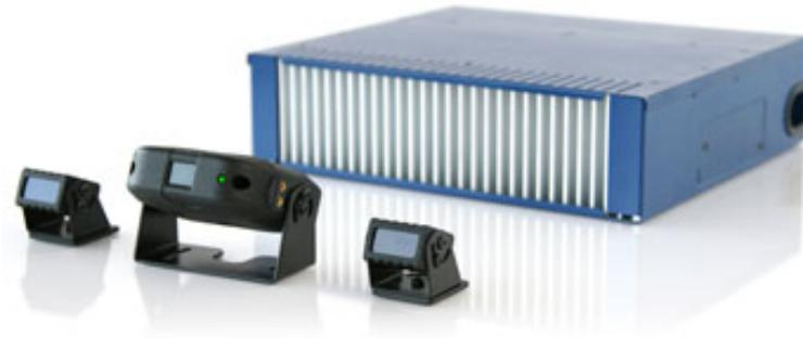
Figura 2.6: DSS (Driver State Sensor)
