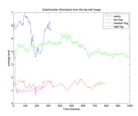
Figure 6: Sobel statistics in various levels of fog
