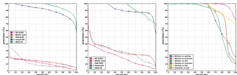
Fig. 3. P-R curves showing the performance of ABLÉ-M in challenging life-long localization scenarios.
