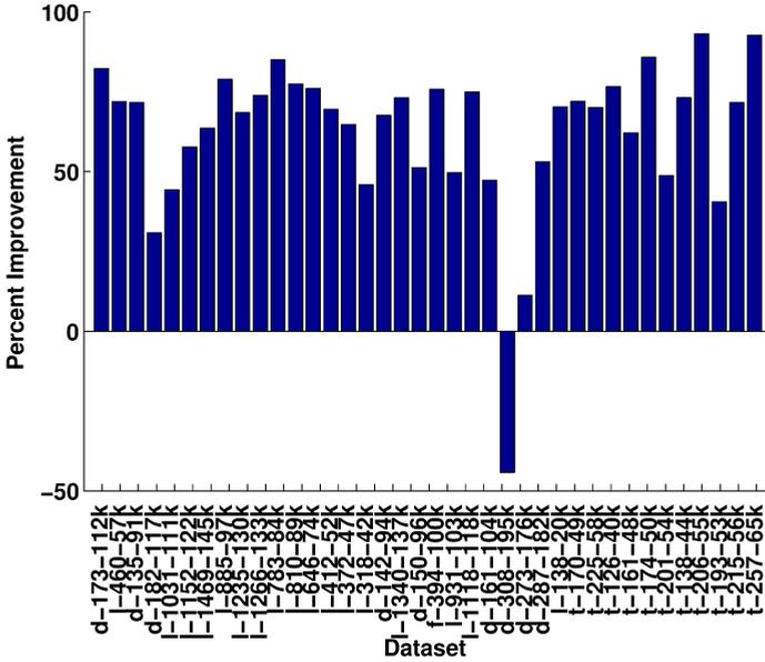
**Figure 4:** Reduction in the average LM iteration time of gCG w.r.t. cCG. Time reduction is computed as  $(T_{\text{cCG}}^{\text{LM}} - T_{\text{gCG}}^{\text{LM}}) / T_{\text{cCG}}^{\text{LM}}$  (%), where  $T_i^{\text{LM}}$  is the average time for a single LM iteration, for technique  $i$ . The only negative peak, for which gCG is slower than cCG corresponds to the dataset d-308-195k, in which Ceres terminates earlier (details in Fig. 5).
