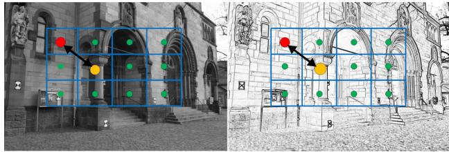
Fig. 1: **Binary descriptor computation.** Given an image patch  $\mathbf{p}$  and a sampling pattern, one bit in the descriptor results from the comparison of image intensities (left) or other image cues such as gradients (right). The sampling pattern can be either fixed or adapted to the dominant orientation and scale.
