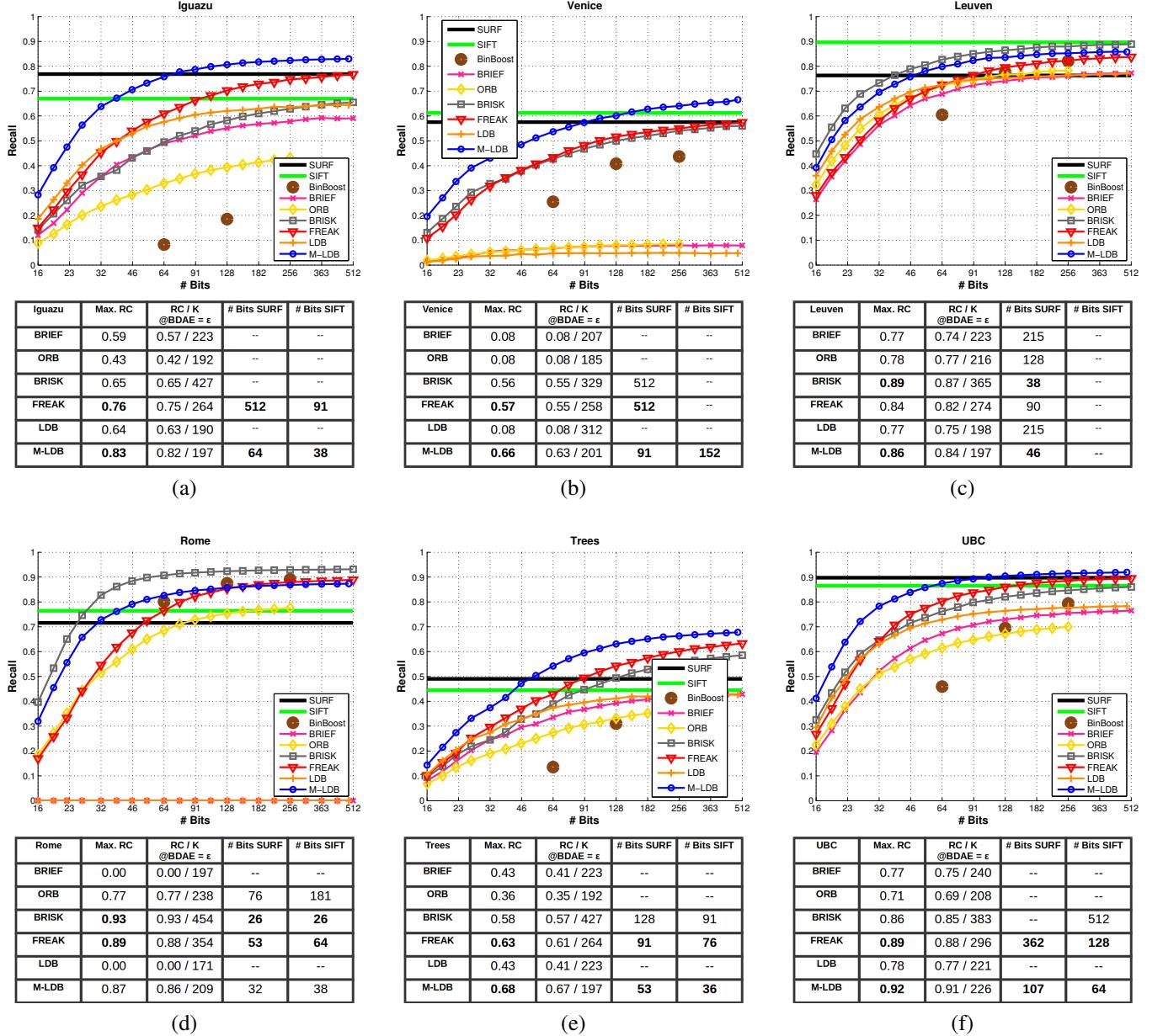
**Fig. 3: Image matching evaluation.** Recall (RC) versus number of bits graphs and statistics for the image matching evaluation. (a) Iguazu (Gaussian noise), (b) Venice (scale), (c) Leuven (lighting), (d) Rome rotation), (e) Trees (blur), (f) UBC (JPEG compression) sequences. Best two global image matching statistics are in bold.
