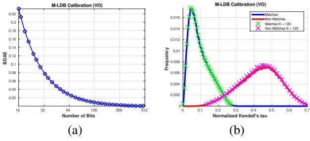
Fig. 5: Local binary descriptors calibration. (a) BDAE for M-LDB. (b) Normalized Kendall's tau histogram and LSH approximation with  $K = 120$ .
