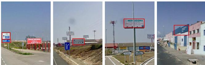
Fig. 8: Panels detection under cluttered background. The two leftmost images are correct detections and the rightmost ones are false positives
