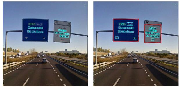
(a) Text detection before panel detection (b) Panels detected and text detection after panel extraction
