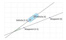
Fig. 9. Heading angle calculation
