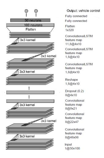
Fig. 4. DeepestLSTM-TinyPilotNet architecture
