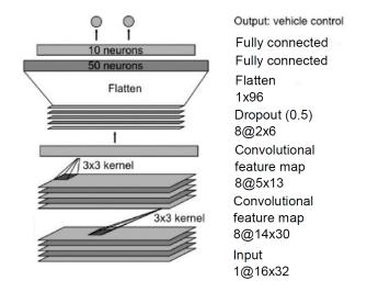
Fig. 2. TinyPilotNet architecture
