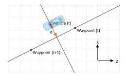
Fig. 8. Distance to the center of the road calculation
