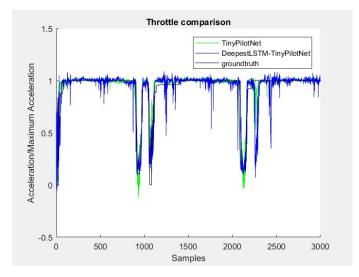
Fig. 11. Throttle frame-to-frame comparison between DeepestLSTM\_TinyPilotNet, TinyPilotNet and human ground-truth
