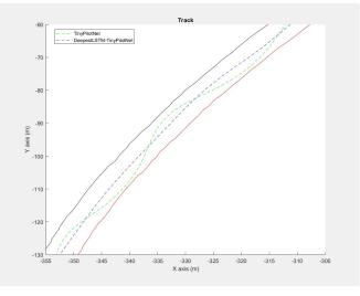
Fig. 12. Fragment of track showing TinyPilotNet and DeepestLSTM\_TinyPilotNet car trajectories.
