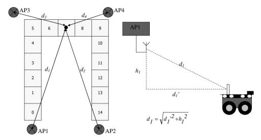
Fig. 8. Example of distance parameter calculation for the seven nodes and AP1.
