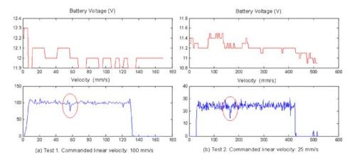
Fig. 5 Vehicle battery voltage and linear velocity during a collision-and-drag case
