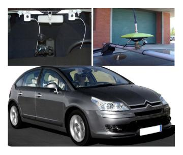
Fig. 2. (Bottom) System architecture mounted on a commercial car. (Top left) Stereo-vision system and low-cost GPS. (Top right) Ground truth RTK-GPS.
