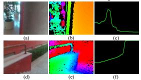
Figure 4. (a)(d) Color images; (b)(e) Depth maps; (c)(f) Traversable lines.
