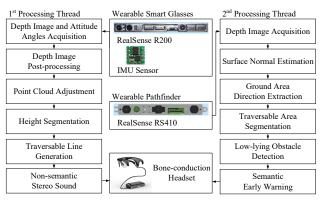
Figure 1. System architecture
