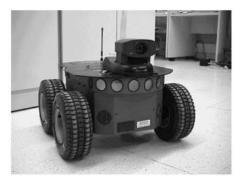
Fig. 4. UAH platform: BART (Basic Agent for Robotic Tasks) robot.
